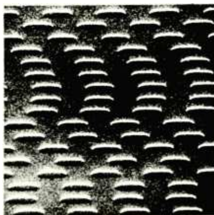
PITS STAMPED IN VLP DISC contain video and audio information. This is a microphotograph of a section of the disc surface.
