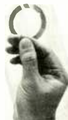
RECORDED DISC used with the i/o Metrics system is on film that can be rolled and handled without harming the recorded information.
