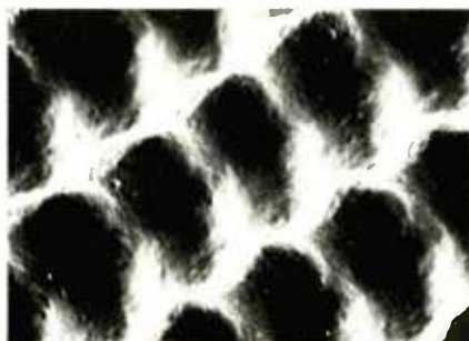
SECTION OF TELEFUNKEN/DECCA MOLDED DISC photographed with a raster-scanning electron microscope. Enlargement is 20,000 times.
